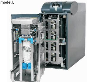
Banknotes' recognition is performed by CIMA's sensor BV 5000 employing all the most advanced technologies: magnetic, infrared, fluorescence, ultraviolet, visible light. It's possible to have both the authenticity recognition function and the fitness feature; in both cases all solutions comply with the regulations of the major National and Central Banks.
